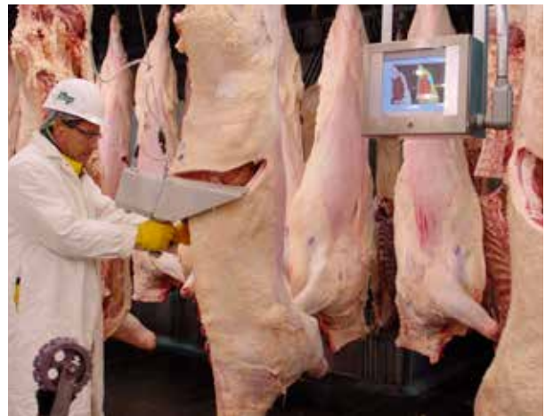
Operation of a computer vision grading system to assess quality and yield of beef carcasses.
